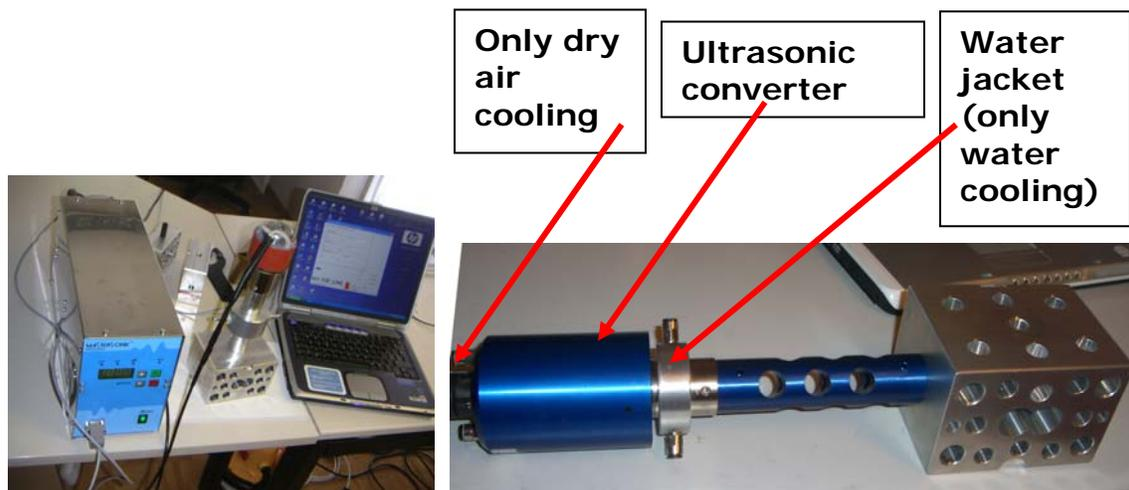
Picture of the complete ultrasonic system configuration: MMM-Generator (left), Converter-Wave-guide-Water-jacket-Aluminum block (middle) and PC (right). PC Interface RS485 to USB (or RS232) is connected between the PC and MMM generator. Client should use his own PC. Software [mpi\\_ix.exe](#) for the MSG.1200.IX should be installed (download software here:
