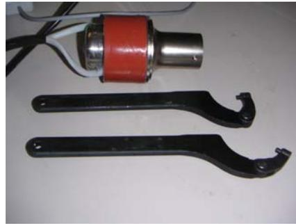
For fixation (screwing, unscrewing) of converter and wave-guide use here presented wrenches.
